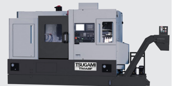
TMA8F featuring five-axis simultaneous control function for machining complex shapes
